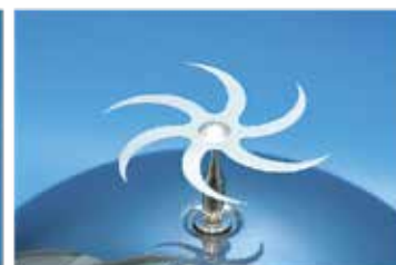
When the Electric Whirl is charged, the discharge repulsion at the point can make the wheel rotates freely on the axle.
