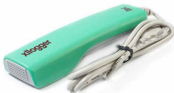
USB Relative Humidity Sensor Xlogger Relative Humidity Sensor. Range: 0 to 100% - Resolution: \pm 0.4\% - Accuracy: \pm 2\% at 25^{\circ}\text{C}
