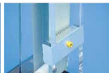
Use the additional comb to optimize the electric charge on the Van de Graaff sphere.
