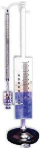
Springs Large Compression- Extension Springs Extension springs. 50 Mm approx. Long, dia 10 mm and wire of 19 SWG.
