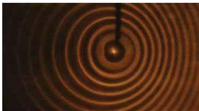
Ripple Tank FGE 13 performing Doppler effect experiments.
