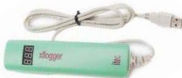
USB Light Sensor Xlogger Light Sensor. Range : 0 - 15,000 Lux
