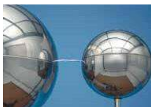
50 - 100 mm length of spark, depending on ambient conditions.
