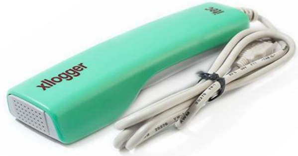
USB Relative Humidity Sensor Xllogger Relative Humidity Sensor. Range: 0 to 100% - Resolution: \pm 0.4\% - Accuracy: \pm 2\% at 25°C
