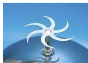
When the Electric Whirl is charged, the discharge repulsion at the point can make the wheel rotates freely on the axle.
