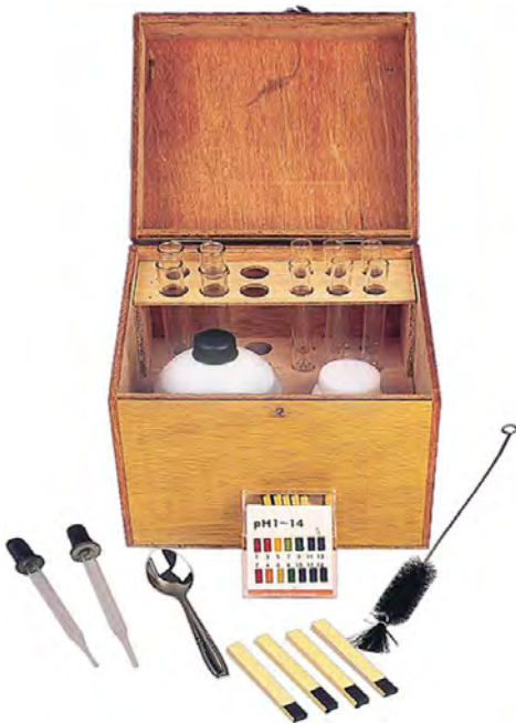
Soil Test Apparatus Use to measure soil pH. Consist of : Test Tube \varnothing 16 x 150 mm 4 pcs Test Tube \varnothing 13 x 100 mm 6 pcs Dropping Pipette 15 cm, Red Bulb 2 pcs Barium Sulphate (100 g/bottle) 1 pc Aquadest (200 ml/bottle) 1 pc Spoon, Stainless Steel 1 pc Universal Indicator (10 booklet/pack) 1 pc Test Tube Brush \varnothing 24 mm 1 pc Manual Book Soil Test Apparatus 1 pc Wooden Box 1 pc Dimension : (L) 20.00 x (W) 19.00 x (H) 19.00 cm Weight : 1.330 kg
