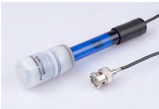
PH electrode The pH electrode 031 is a gel-filled Ag-AgCl combination-electrode in a plastic tube. It has a coax cable, with a BNC connector. It is supplied in a bottle filled with a protective solution. The electrode cannot be refilled.
