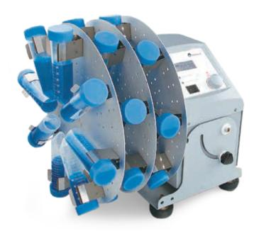
ES rotators give gentle but effective mixing of biological samples held in 1.5mL to 50mL tubes, and are used in a variety of applications including immune precipitations, prevention of blood coagulation, latex diagnostics, etc.
