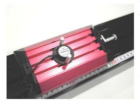
The supplied fasteners are used to attach devices to the cart. For example, you may want to attach a force sensor, accelerometer to the cart. The fasteners may be inserted any point along the slot length. To use, loosen but do not remove the nut from the shaft, and insert the nut parallel to the slot. Turn the shaft clockwise to tighten.
