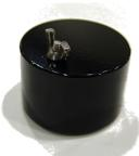
The 500g mass is used to double the mass of the cart. Attach the mass by removing the wing nut and bolt, and placing the bolt head in one of the off-center slots on top of the cart. Slide the mass over the bolt, and tighten the wing nut.
