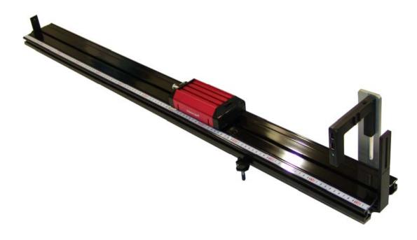
The Dynamics system consists of a 1.2m track, two carts, and related accessories. The system is designed for use in physics and physical scientific experiments. Dynamics system enables more accurate and precise experiment by minimizing friction. Some typical experiments done with the system include
