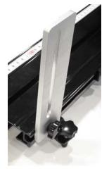
Photogate bracket is attached to the side of the track. With the nut loosely on the T-handled bolt, slide the nut into the side channel of the track. Attach the photogate using the supplied wing bolt in the long slot. Adjust the gate height so the beam intercepts the desired portion of the target.
