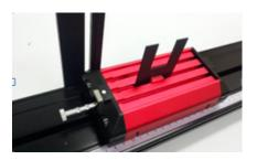
To study totally inelastic collisions, change polarity of one cart to be opposite each other. This way any cart will stick to any other. Carts with magnets will stick together, creating a totally inelastic collision.
